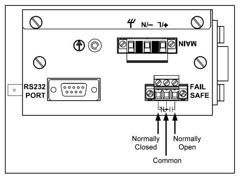
Figure 7 - RS910L Failsafe Output Relay
